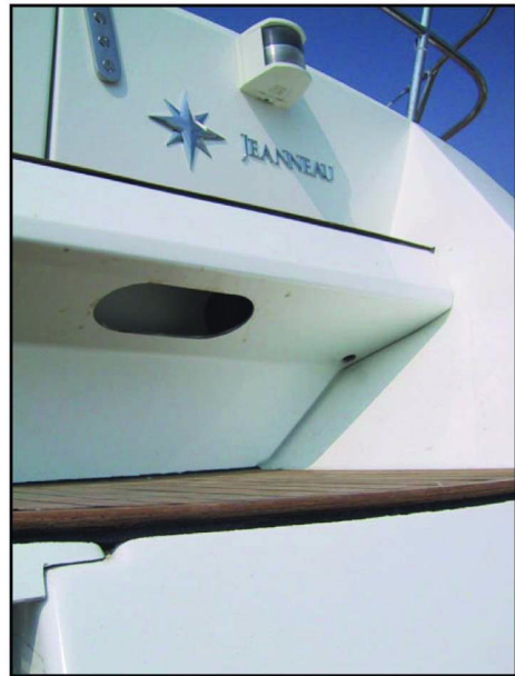
Engine compartment bilge ventilation
