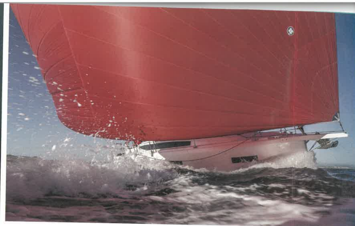
ABOVE Plenty of breeze and the bow is forced down, immersing the fuller hull sections and giving the boat extra power
