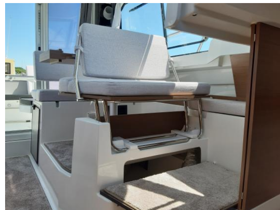
Copilot bench : very easy to transform into saloon bench by simply tilting the backrest
