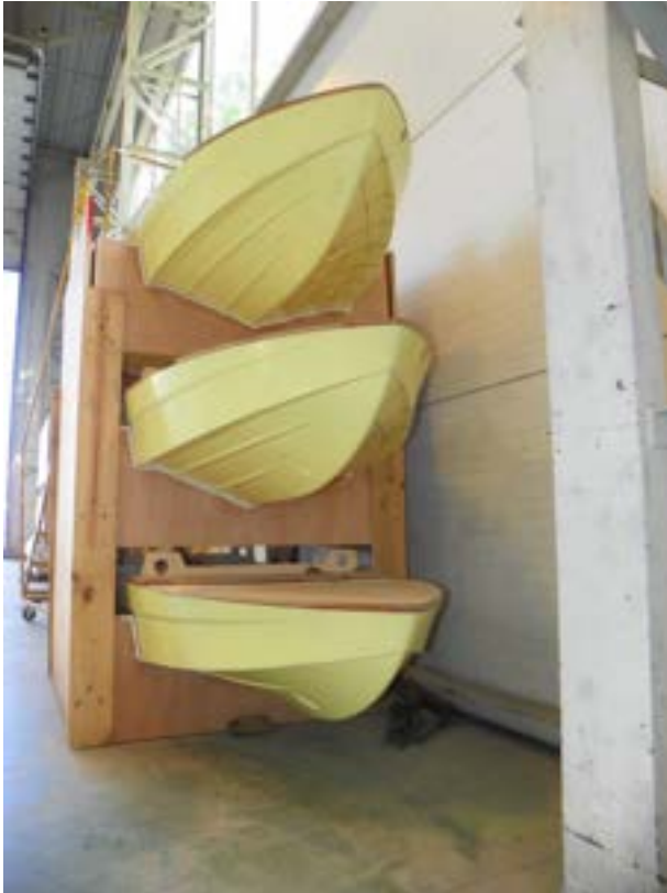
NEW HULL OPTIMIZED FOR OUTBOARDS AND FLAT CRUISING AT INTERMEDIATE SPEEDS, IN THE SAME SPIRIT AS THE HULL DEVELOPED FOR THE MERRY FISHER 1095.
