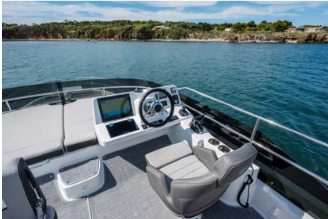
Cockpit with full instrumentation for engine and accessories (same as inside instrumentation)
