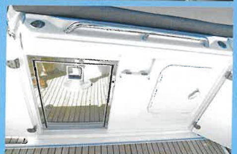
1. A hidden windlass and remote controller. 2. A clever feature that gives easy access to the forecabin. 3. The fridge sits behind two doors.
